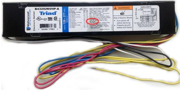
A typical Non-PCB containing fluorescent light ballast. The ballast has a "No PCBs" marking on the top of the ballast and the text "electronic ballast". Only magnetic fluorescent light ballasts contained PCBs.
